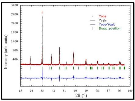
Fig. 1: The X-ray diffraction pattern of the powdered sample at room temperature using Cu-K<sub>α</sub> radiation is shown.
