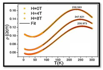
Fig 3: Resistivity (ρ) vs. temperature (T) plot of the sample at 0, 4, and 8T magnetic field, where solid lines show the fitting carried out with the combined  $\rho_{FM}(T)$  and  $\rho_{PM}(T)$  respectively, using eq. 9.
