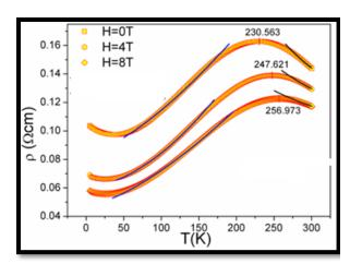
Fig 2: Resistivity ( $\rho$ ) vs. temperature (T) plot of the sample at 0, 4, and 8T magnetic field. The fitted line shows fitting to the empirical model for T<T<sub>MI</sub> and the variable range hopping model for T>T<sub>MI</sub>.
