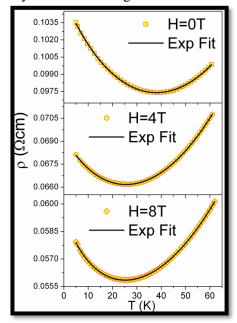
**Fig. 4:** The low-temperature resistivity data with different magnetic fields. A solid black line represents an experimental fit.
